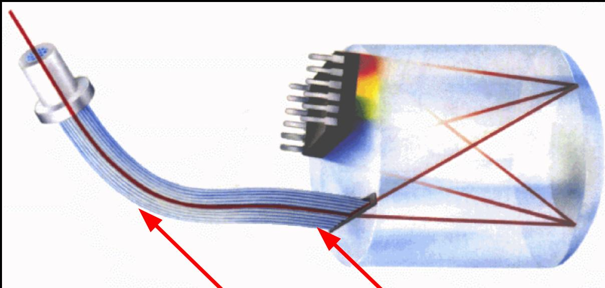
**Monolithic diode-array monochromator:**
