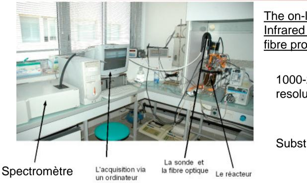
The on-line monitoring by Near Infrared Spectroscopy with a fibre probe.
